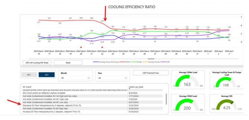
Key lesson: Measure and validate all energy efficiency efforts; increasing IT equipment inlet temperatures does not guarantee efficiency improvement – it is dependent on the overall system characteristics
