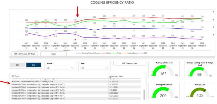
On September 18th, the IT space temperature was increased from 74°F to 75°F. CER decreased from 4.08 to 3.67. CRAH energy consumption increased from 193 to 217 kw. Chiller energy consumption increased from 168 to 199 kw
